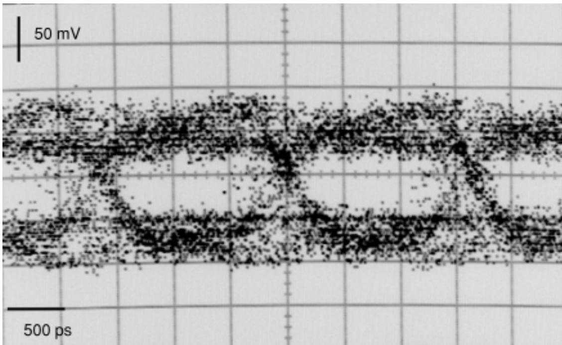
Figure 10. Eye diagram for an ultra-thin silicon on sapphire CMOS optoelectronic receiver circuit.
