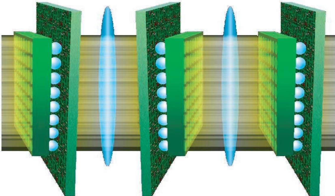
*Figure 2. Parallel interconnect cascade information processing architecture employing through-the-substrate optical vias and high-speed CMOS processing circuits.*
