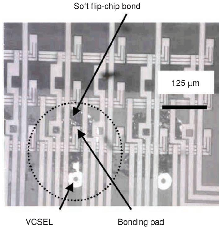
Figure 8. Photograph of the integrated module taken from the backside of the SOS CMOS die.
