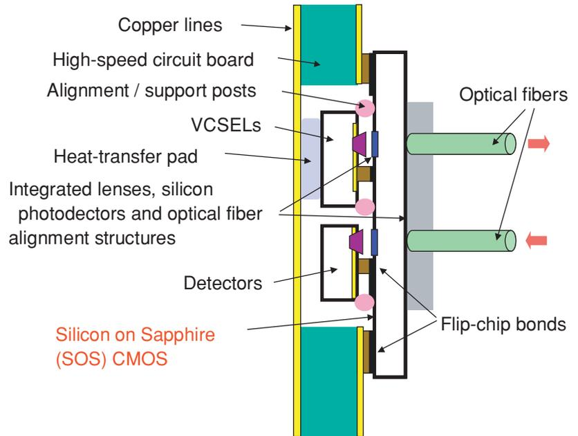
Figure 1. Die-as-package optoelectronic module comprised of a silicon on sapphire CMOS die, active photonic elements (detector and VCSEL arrays) and passive photonic waveguides and couplers that direct light into bundles of optical fibers.
