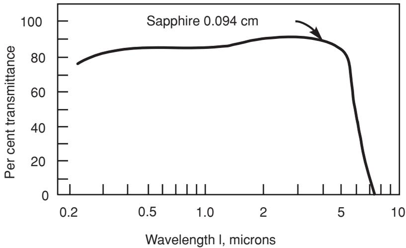
Figure 3. Optical transmittance of sapphire (adapted from [6]).
