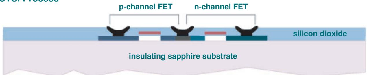
Figure 4. Ultra thin silicon on sapphire CMOS process compared to a standard bulk CMOS Process.
