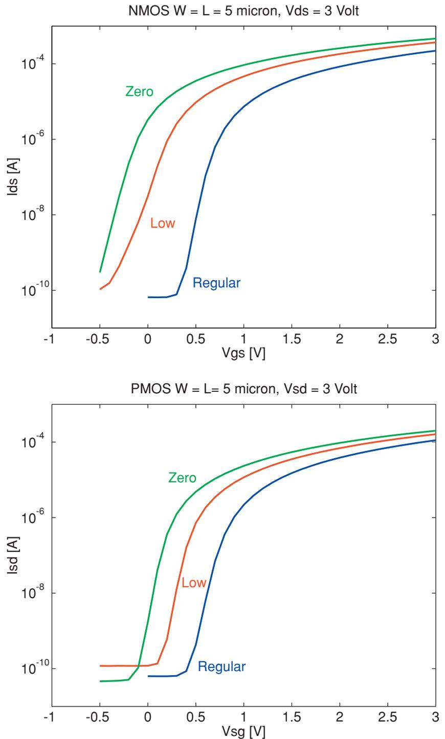
Figure 5. Typical transfer characteristics for the six types of three terminal devices available in the Peregrine SOS process.
